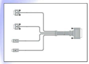
FIGURE 2 CA-100872 Cable for connection to each PC
